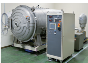
Vacuum Tolerance Testing Chamber 真空試験槽
