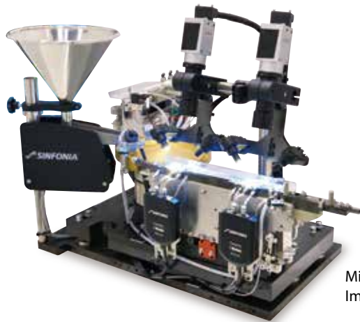
High Frequency Mini Parts Feeder unit for chip LED
